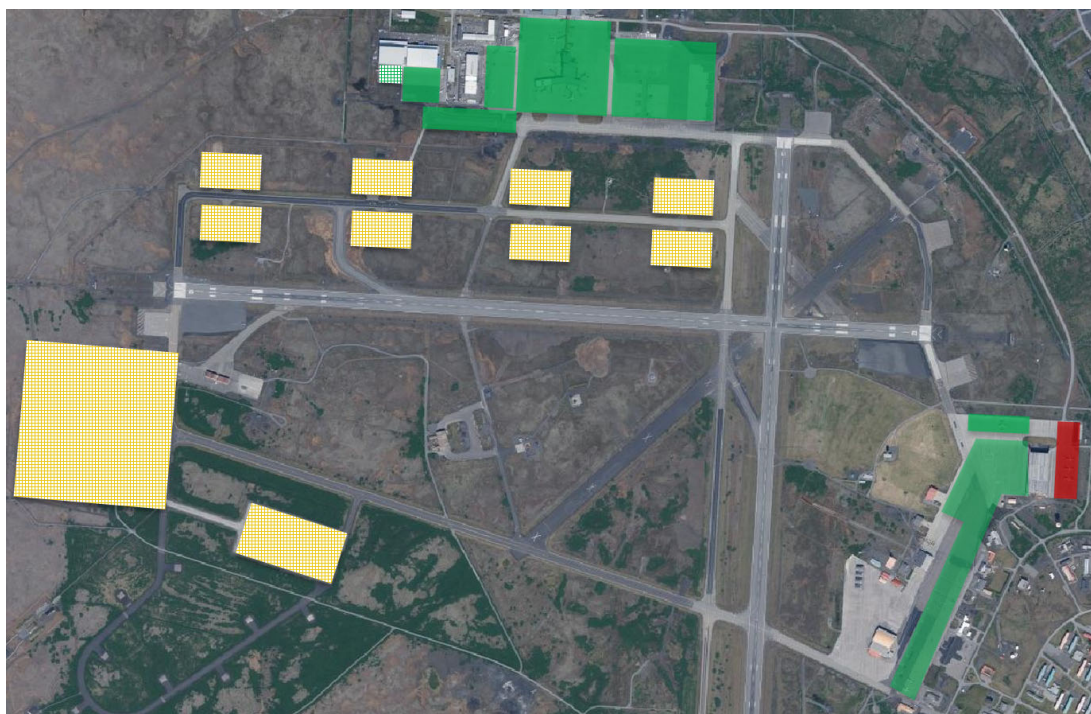
Figure 2. Apron priorities. The green areas are serviced on a daily basis. The yellow ones are serviced on demand in collaboration with APOC and The Coast Guard. The aircraft stands in red east of hangar 885 are closed during winter.
